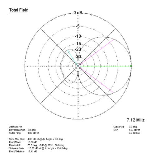
Peak Gain is shown over a dipole in Freespace Dipole in Freespace = 2.14dBi
